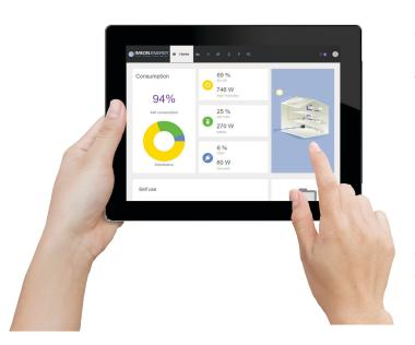
With an intuitive interface developed in HTML 5, the IMEON MANAGER application can be accessed on any device and allows to follow your installation in real time! The application has different tabs allowing you to visualize the information concerning the energy produced by the photovoltaic system, energy stored in the battery and characterizing the public electricity distribution network. A historical data is easily available and configurable.
